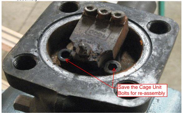
5. Remove the Cage Unit inspecting seating faces for wear or damage
