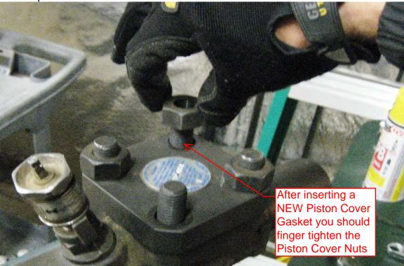
22. When you are certain ALL steps have been completed successfully, tighten the **Piston Cover Nuts** evenly in a diagonal pattern until you reach the desired torque of 60 ft-Lbs for the SPF0-3 (100 ft-Lbs for the SPF4-7)
