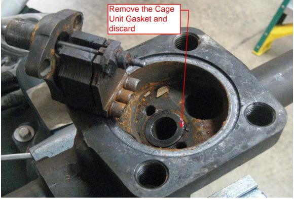
7. Insert the **NEW Cage Unit Gasket** making sure the area is clean of dirt and debris
