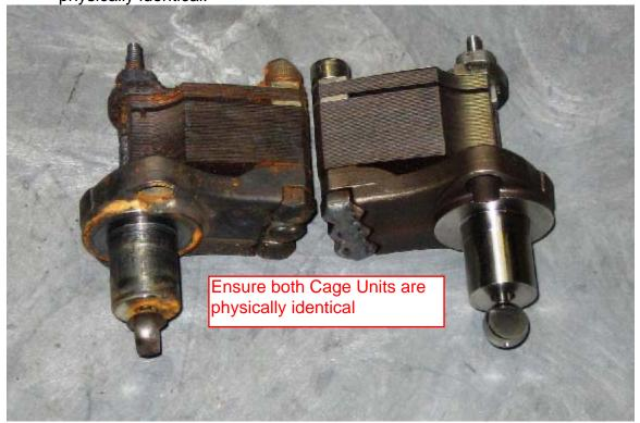
9. Insert the **NEW Cage Unit** into the trap carefully aligning the slotted valve assembly with the temperature controller. Make sure that the bimetal plates are clean and that the space between the segments is clear.
