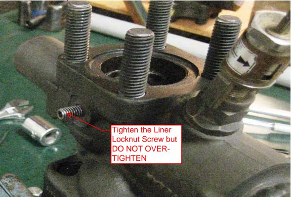
20. Install a **NEW Liner Locknut Gasket** and secure the **Liner Locknut** to prevent loosening of the **Liner Locknut Screw**.
