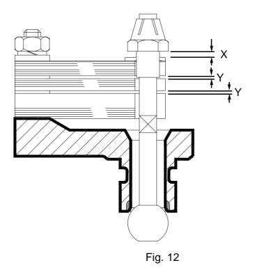
The clearance is measured at point 'X 'Fig.12 between the top of the rocker plate and the underside of the adjusting nut. The standard factory setting is made at an ambient temperature of 65 Deg F (18 Deg C) and will allow the valve to commence opening at 15 Deg F (8 Deg C) approx. Below saturation, with full discharge, as shown in the individual capacity diagrams for each model, around 40 Deg F
