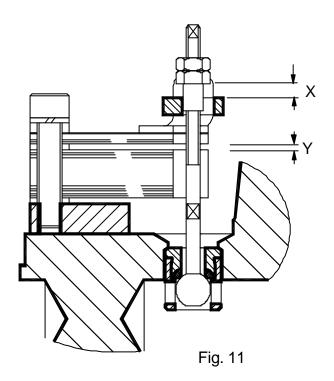
The clearance is measured at point ' X ' fig.11 between the top of the rocker plate and the underside of the adjusting nut. The standard factory setting is made at an ambient temperature of 65 Deg F ( 18 Deg C ) and will allow the valve to commence opening at 15 Deg F ( 8 Deg C ) approx. Below saturation, with full discharge, as shown in the individual capacity diagrams for each model, around 40 Deg F (22 Deg C).
