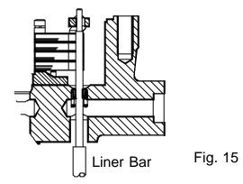
For models N-600/675/900/1500 a multi diameter liner bar is available. This is used from above the trap. Lift out of the rocker plate from its support bridge. Pass the liner bar down the bimetal slot until appropriate diameter is fully inserted into the orifice. Tighten the holding screws, remove the liner bar and replace the rocker plate.
