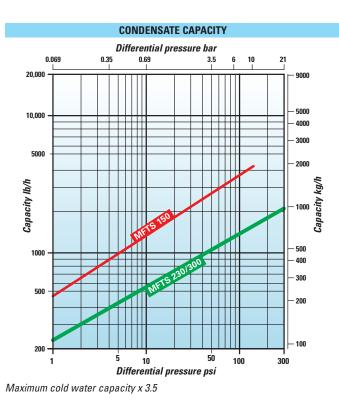
The performance graph indicates the continuous discharge capacities of condensate per hour at various pressure differentials across the trap.
